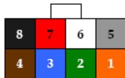
5.4.1 Figure - MARCUS® 3G Radio Connector Pin Layout
