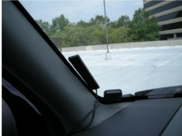
3.3.1 Picture - Example Placement of Glass Mount GPS and RF Antennas
