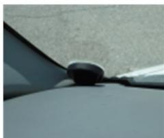
\* Sample of the antenna installed on the windshield. Always make sure window is clean before adhering to glass.
