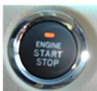
\* *Never* connect directly to the wires on a Push-Button start switch. This may cause damage to the vehicle's BCM. Connect the power and ignition wires to the back of the fuse box or another safe location.
