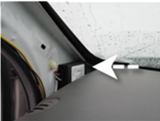
\* Sample of the VTU installed in the "A" pillar of a vehicle. Note how the "white" label is facing out. This is key as the internal GPS receiver is located there.
