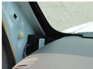
\* Sample of the SQ4400 installed in the "A" pillar of a vehicle. Note how the "white" label is facing out. This is key as the internal GPS receiver is located there.
